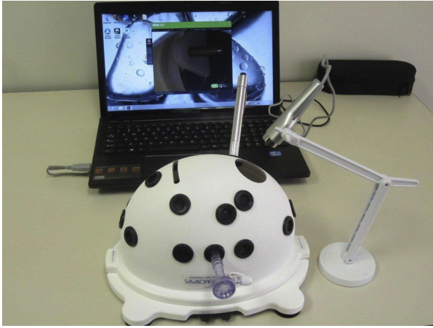
Fig 3. AANA Fundamentals of Arthroscopic Surgery Training workstation with multiple potential portal sites in an opaque dome covering a mandrel around which knots are tied through an arthroscopic cannula (inset on laptop screen). A USB camera (Ipevo, Sunnyvale, CA), directed through a window, projects an image of the inside of the dome onto a laptop computer screen.
